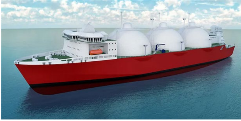
FIGURE 10 Rendering of concept design for a 20,000-m 3 LH 2 carrier (source: Shell/Houder).
