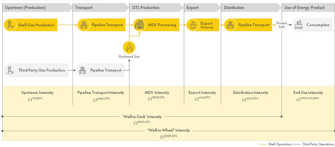
Figure 9: Schematic of the pathway for GTL.
