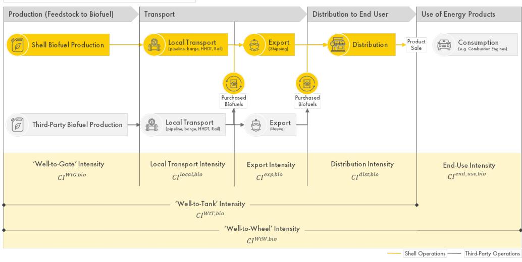
Figure 10: Schematic of the pathway for biofuels.
