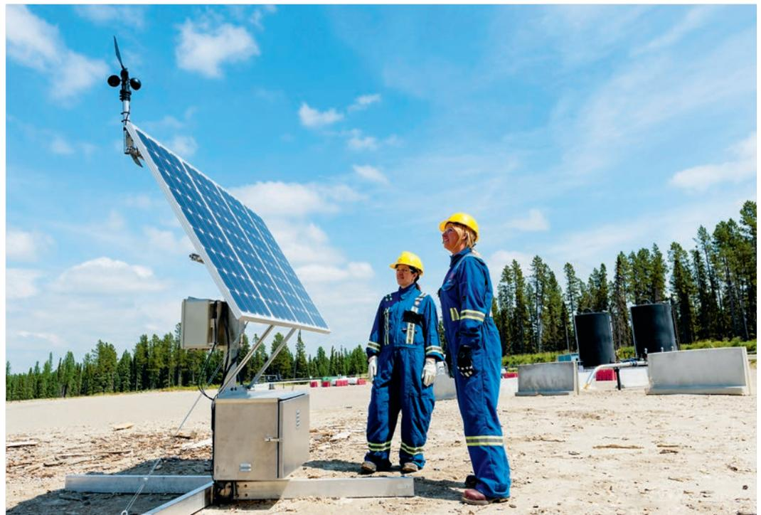
Workers look at methane detection technology during a test at an unconventional gas well in Canada.
