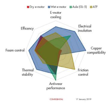
One need that both wet e-motors and dry e-motors share is fluids that offer antifoaming qualities. As OEMs design more compact motors to save weight and space, there are higher rotational speeds to contend with. Increasingly, this means that more electric vehicles will need transmissions to manage the high RPMs of the motors. But the high-stress environment of these transmissions can allow air to get into them and cause fluids to foam, which means
