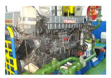
A used oil analysis programme along with expert diagnosis from a local Shell laboratory showed that the oil-drain interval had been safely extended to 1,000 hours from the 700 hours when using a competitor's oil; a 43% increase. In addition, the vessel also improved its operating efficiency through less downtime.
