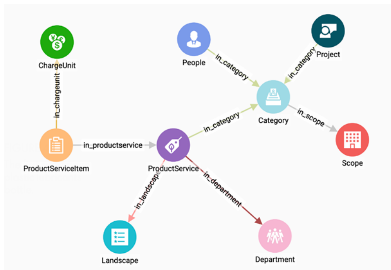
FIGURE 2 The conceptual data model. Image courtesy of TigerGraph.
