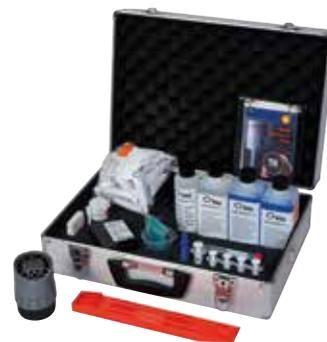
Shell Onboard Plus: measurement of total base number (TBN) and water content
