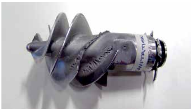
FIGURE 1: Erosion damage to a pump.
