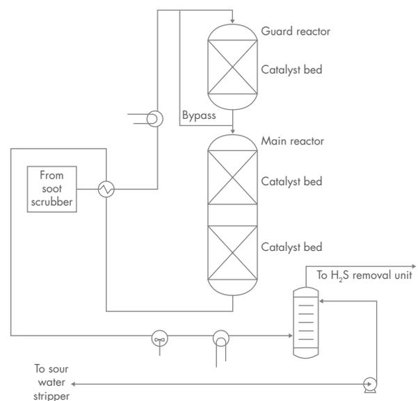
Figure 1: Simplified process flow scheme.
