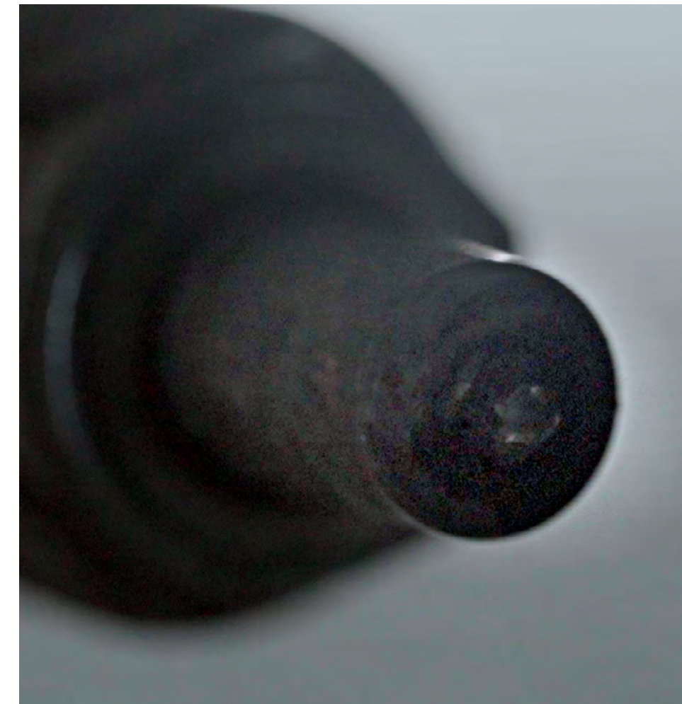
Carbon deposits on injectors using regular diesel.
