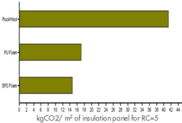
The EPS and PU production process (normalised for the same insulation value per m<sup>2</sup>) results in less than half the carbon footprint compared to Rockwool
