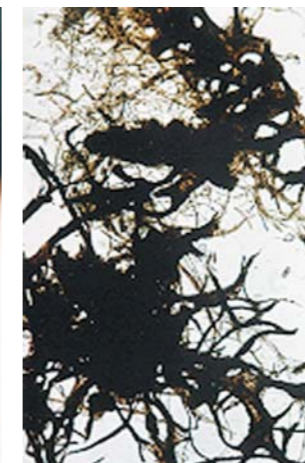
Fungal hyphae and other debris from the surface of a diesel fuel filter which blocked in service.
